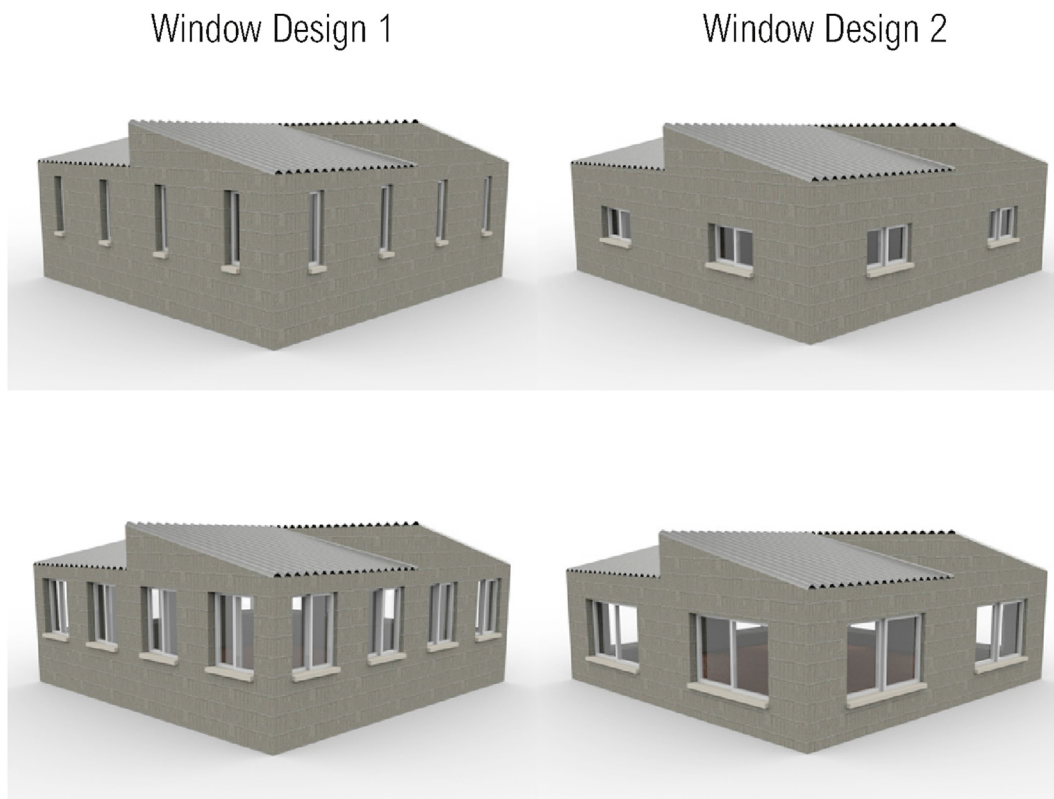
Fig. 5 Window design 1 and 2 with 0.1 (top) and 0.3 WWR (bottom).
