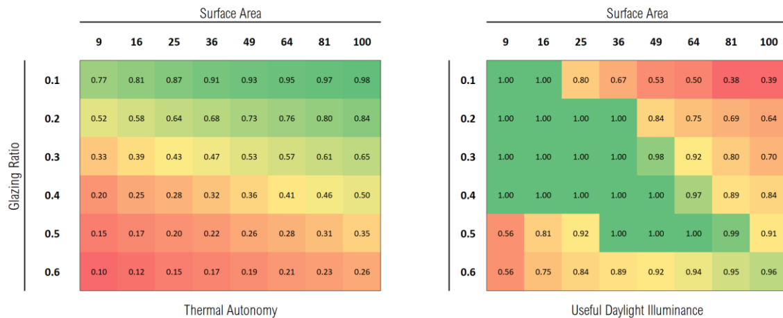
F59 – Thermal Autonomy (left), and Useful Daylight illuminance (right) heatmaps of 'Ventoinha' house with defined design parameters.
