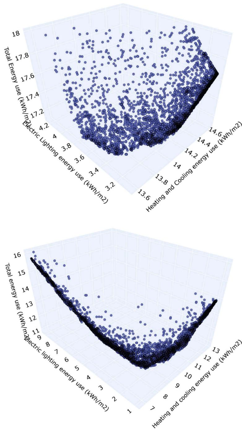
Fig. 7. Tested solutions with NSGAI1 for Copenhagen (Top) and Lisbon (bottom). Results for each objective (x- and y-axis) and the sum of both objectives (z-axis).
