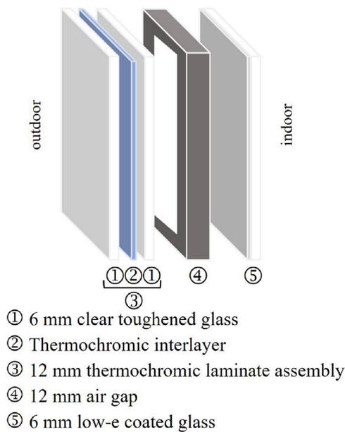
Fig. 3. Thermochromic glazing layers.
