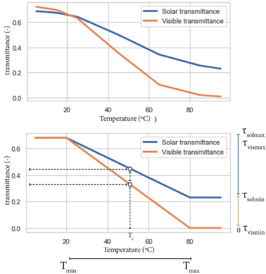
Fig. 4.  $\tau_{sol}$  and  $\tau_{vis}$  values of Thermochromic glazing at different temperatures for one simulation (Top). Approximated  $\tau_{sol}$  and  $\tau_{vis}$  values for simulations for the optimization problem (Bottom).
