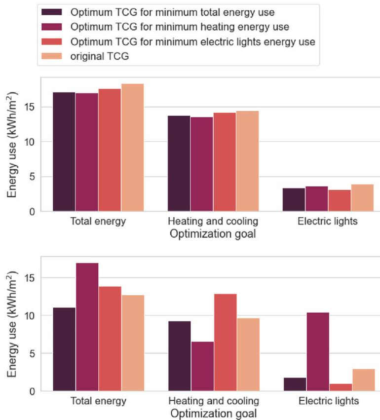
Fig. 8. Office energy use for the Optimum thermochromic glazing of the proposed goals. Comparison with the original in Copenhagen (Top) and Lisbon climate (Bottom).
