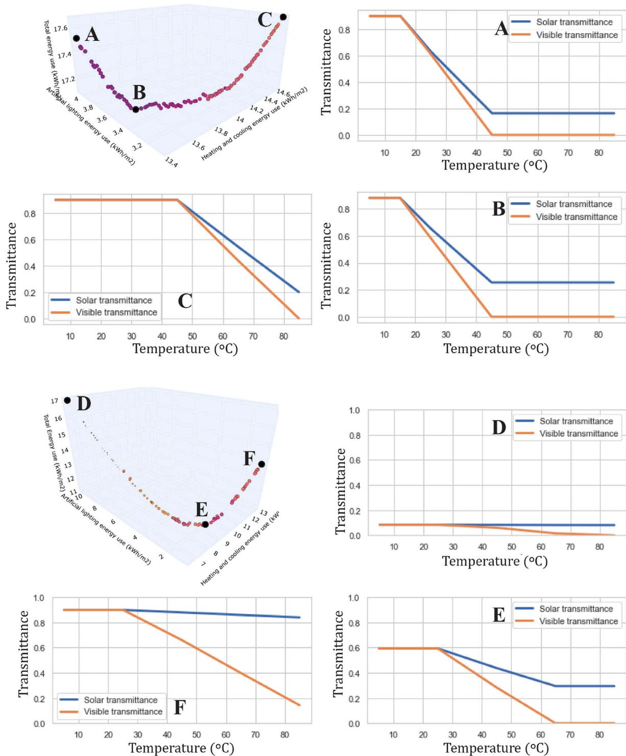
Fig. 10. Thermochromic glazing properties for each optimal solution in both climates. Copenhagen: (A) minimum heating and cooling needs, (B) Minimum total energy needs, (C) Minimum lighting needs; Lisbon: D, E, F, respectively.
