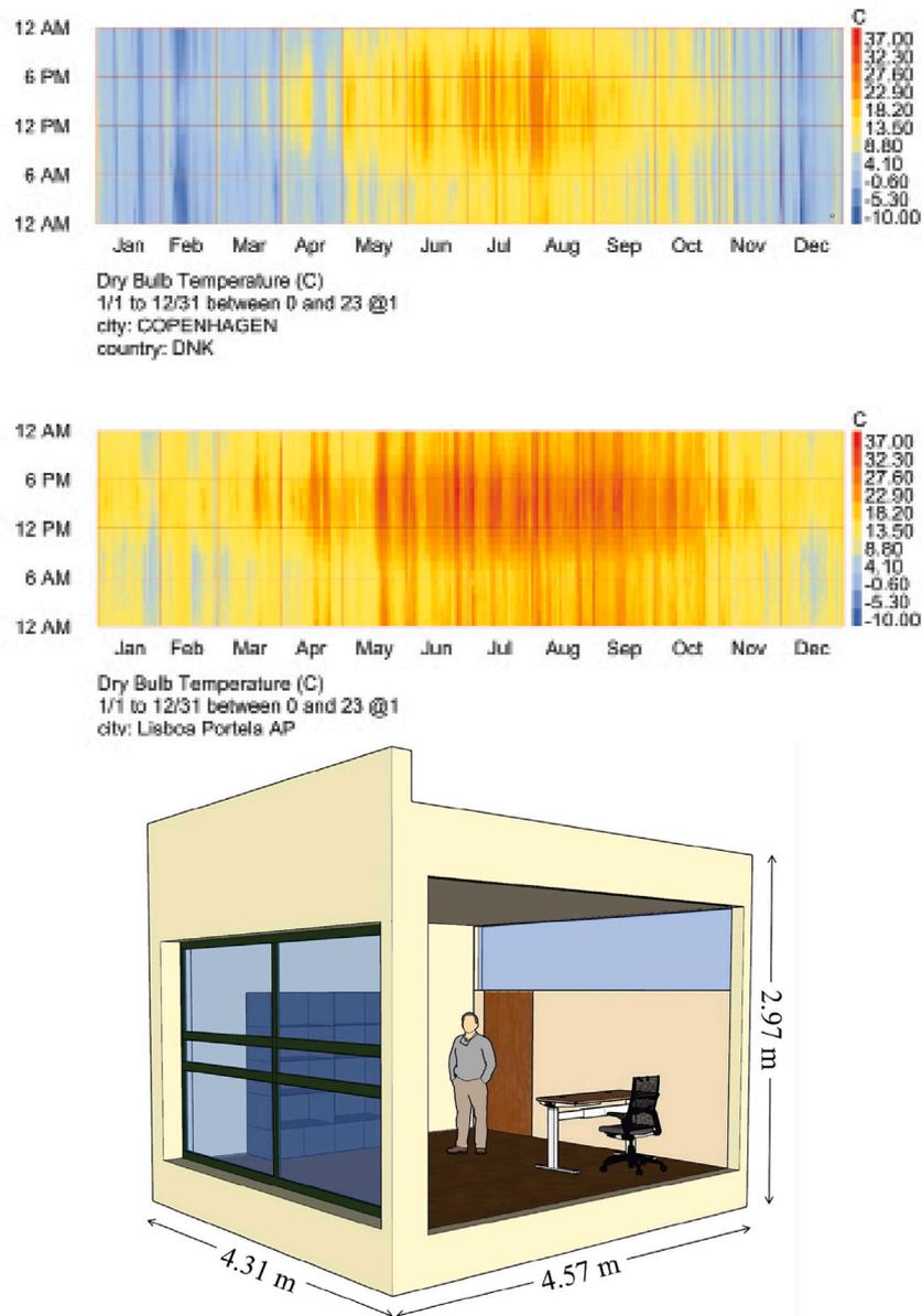
Fig. 2. Top — Denmark (top) and Lisbon (bottom) yearly dry bulb temperature. Bottom — 3D model of the office room used as a case study.
