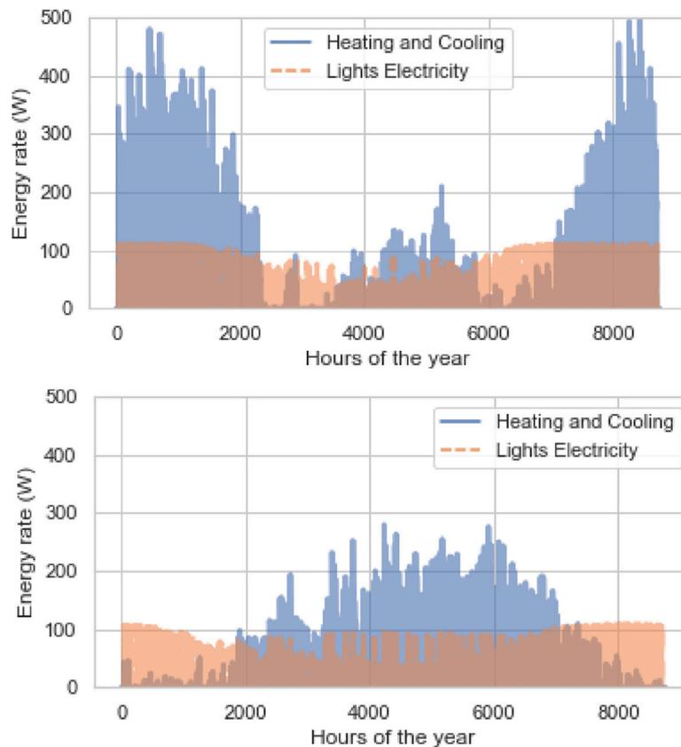
Fig. 6. Hourly heating and cooling, and Electric lighting Rate for Copenhagen (Top) and Lisbon (Bottom).
