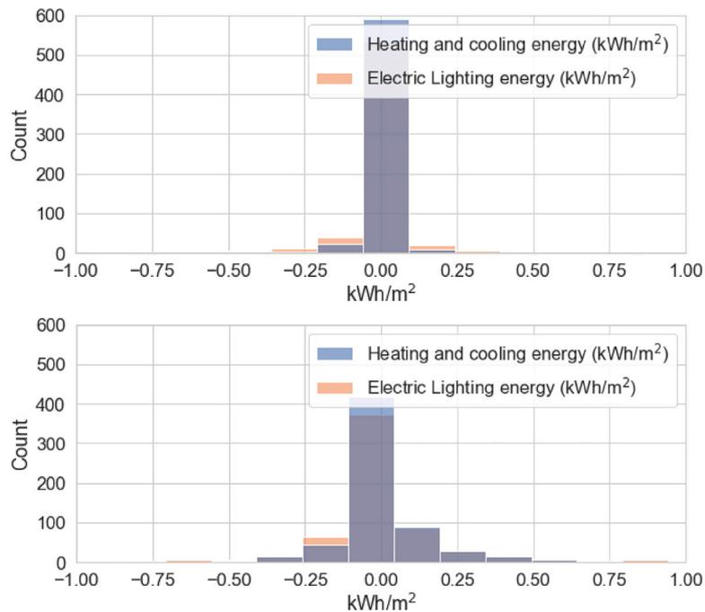
Fig. 5. Error value distribution plot for the test sample in Copenhagen's climate (Top), and Lisbon (Bottom).
