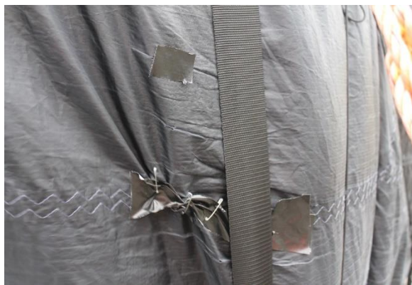
Fig. 3 - Temporary mend of the envelope shreds with tape and safety pins
